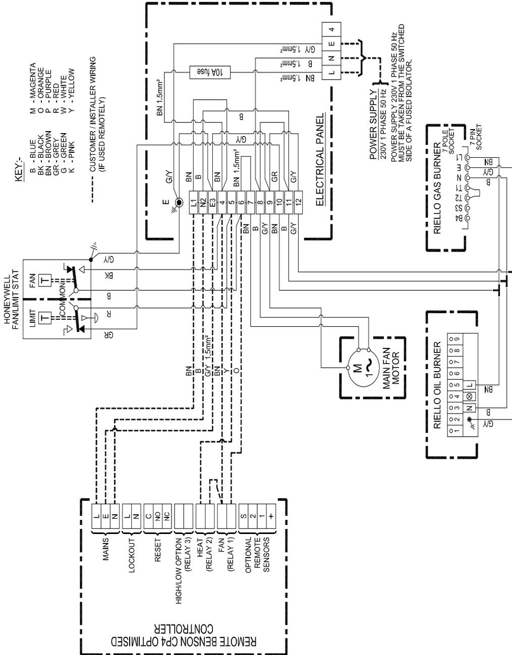
**100 – 300 Riello ON / OFF Gas or Oil Fired Burner
