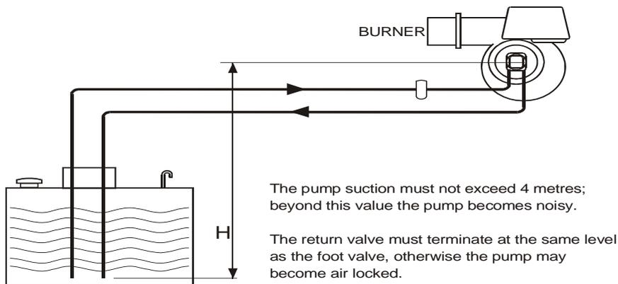
Burner oil pump details 700-1300 suction feed
