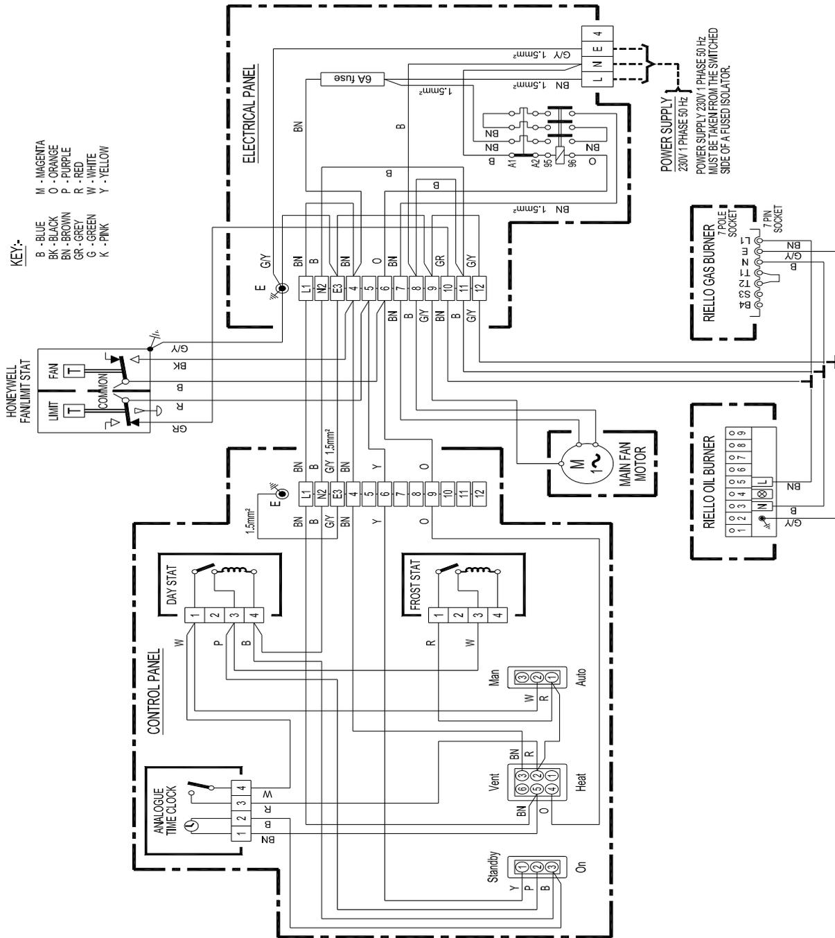
**400 – 500 Riello ON / OFF Gas or Oil Fired Burner
