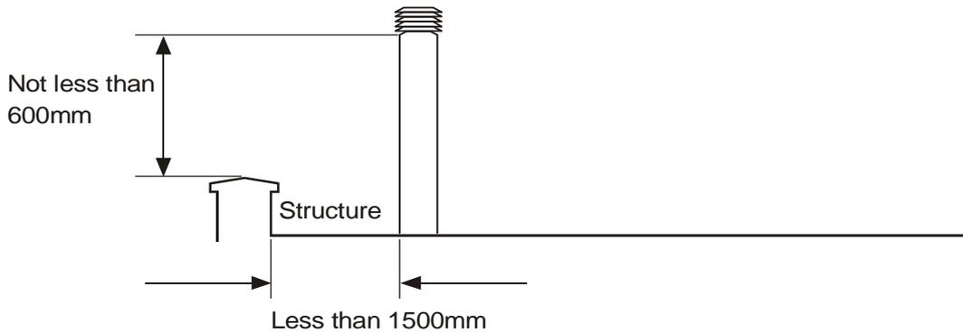
Flat roof with flue close to parapet
