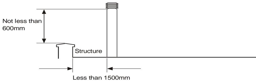
**Fig 5** Flat roof with flue close to parapet
