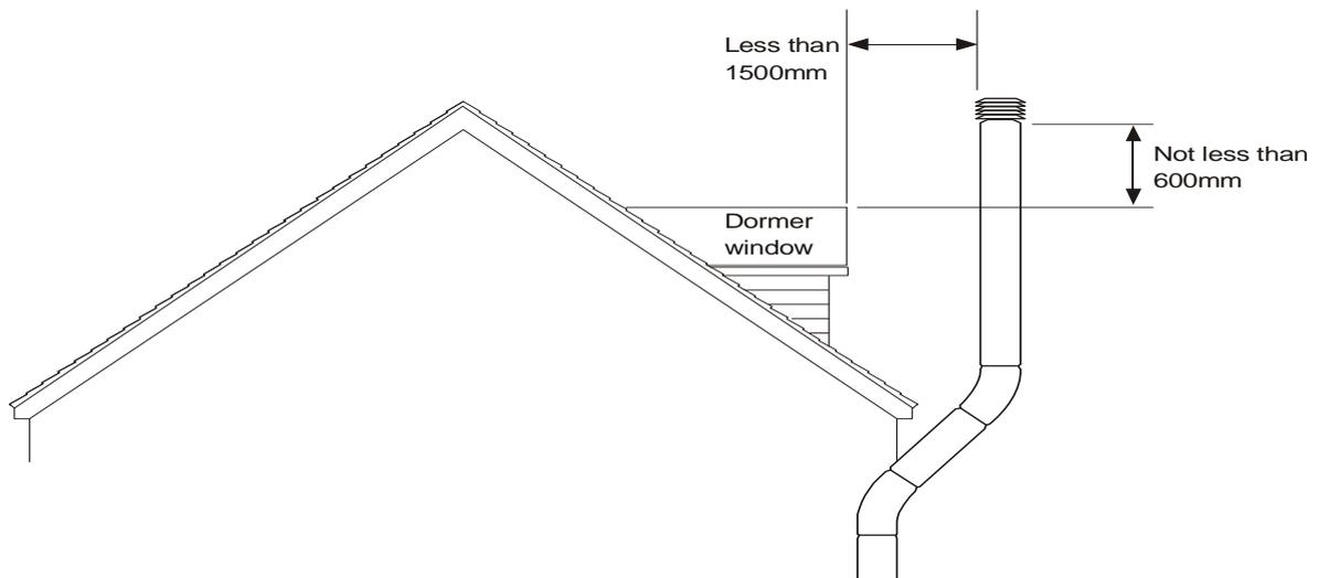
**Fig 9** Pitched roof chimney within 1.5m from dormer window measured horizontally
