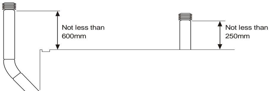
**Fig 6** Flat roof with no parapet
