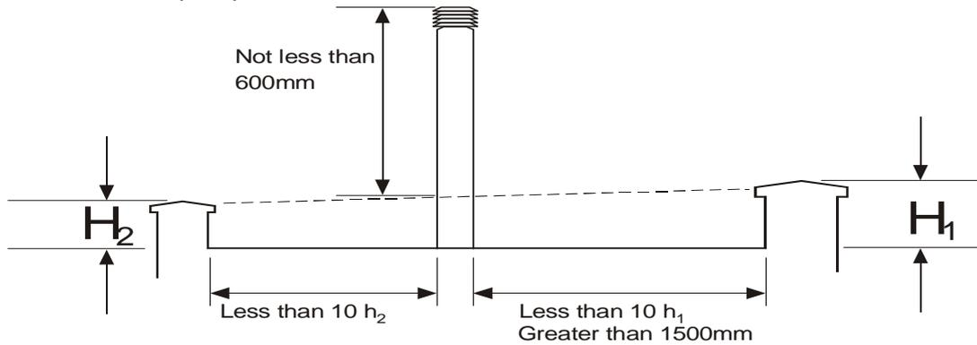
**Fig 3** Flat roof envelope method
