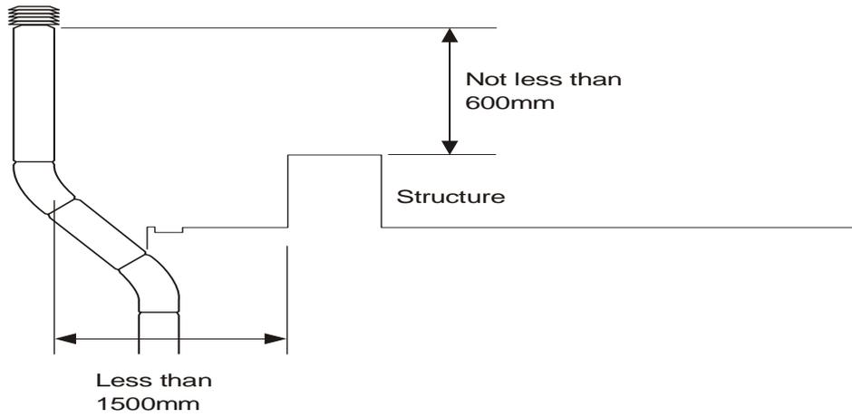
**Fig 7** Flat roof with structure close to flue outlet
