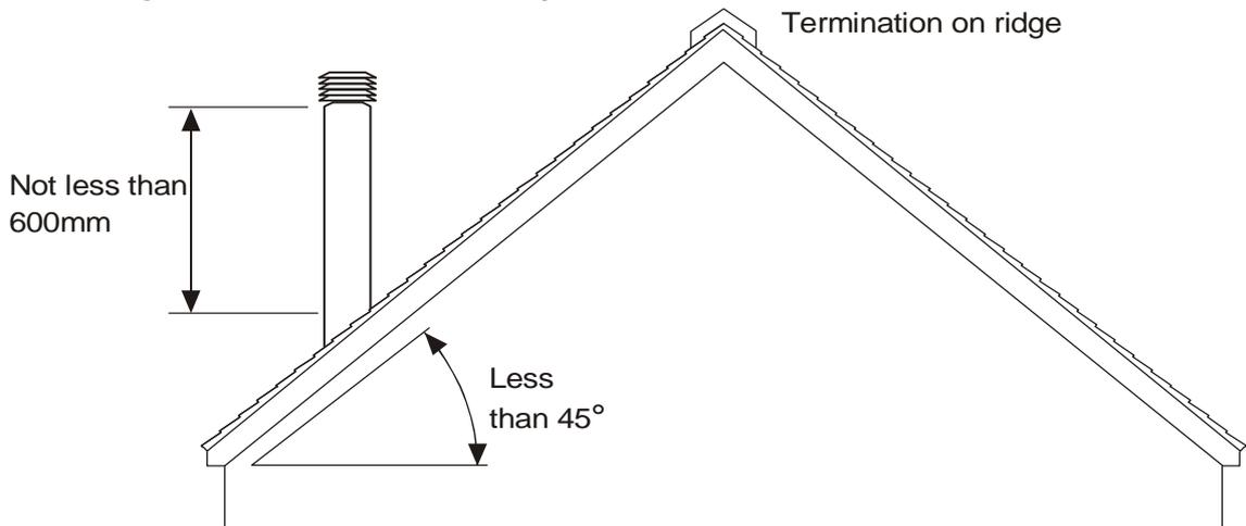
**Fig 11** Pitched roof internal route not exceeding 45° and ridge termination
