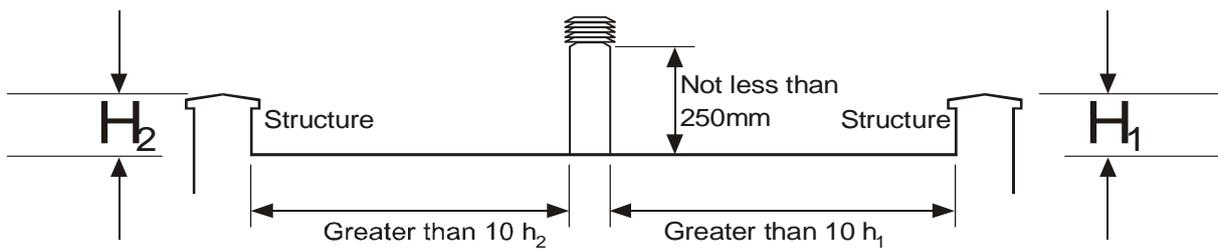
**Fig 4** Flat roof where the flue height is more than 10 Heights ( $H$ ) away from all structures
