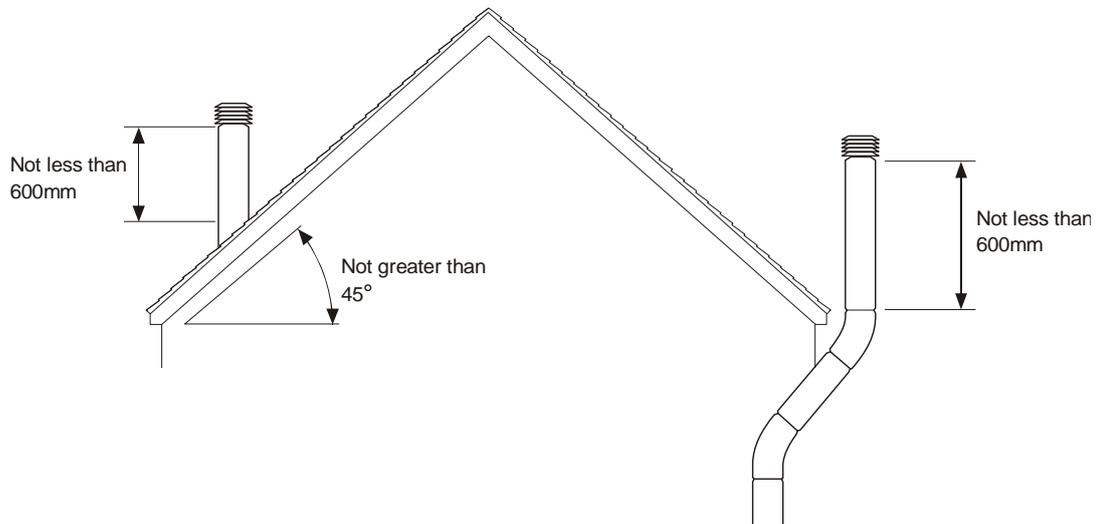
**Fig 8** Pitched roof not greater than 45°
