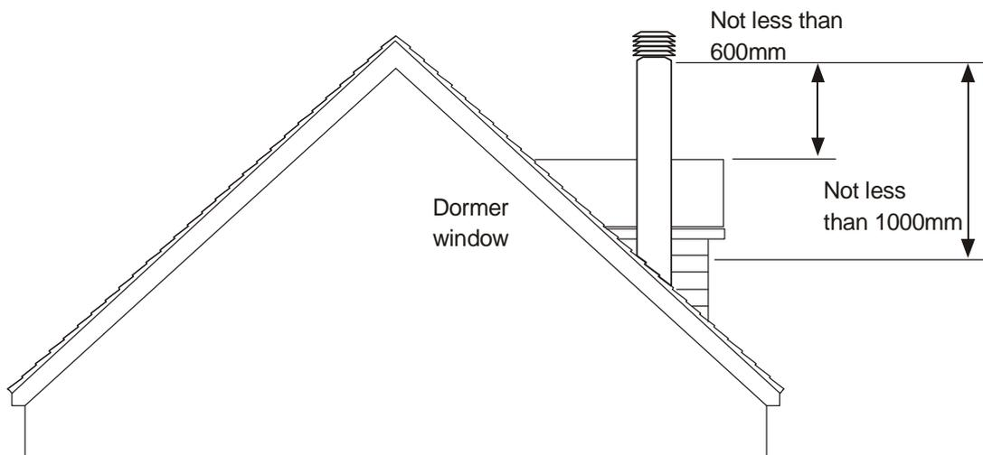
**Fig 12** Pitched roof chimney within 1.5m from dormer window measured horizontally
